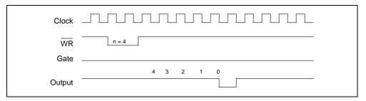
**Figure 2-36.** Mode 4 Timing Diagram
